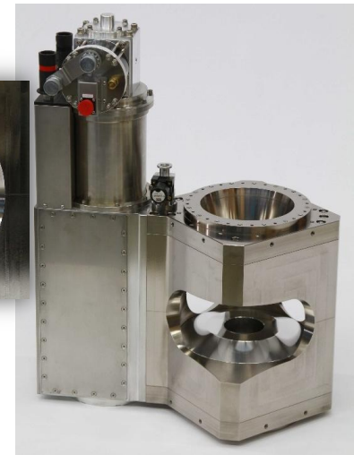
2.2T Instrument magnet - TOFTOF
