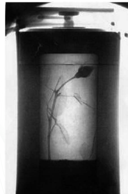
Neutron Radiograph of Rose in Lead Flask
