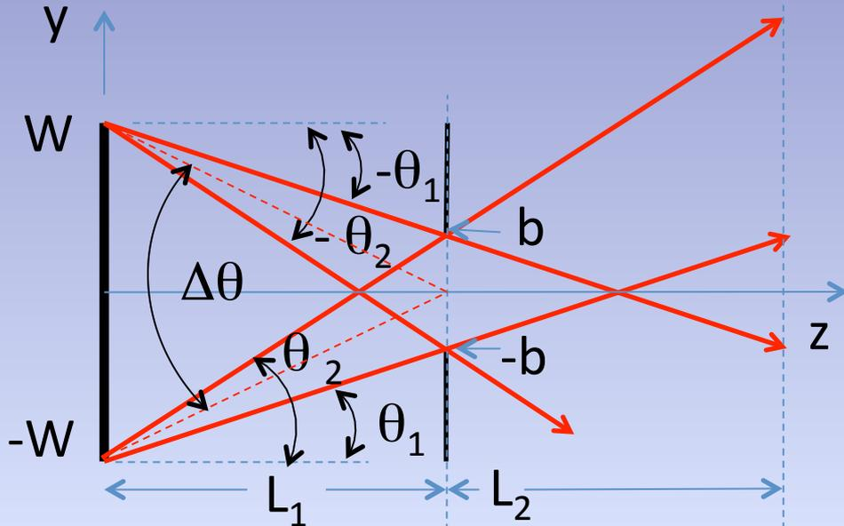
Propagating in real space produces a shear of the phase space diagram. Area of phase space is constant and the phase space density is constant.
