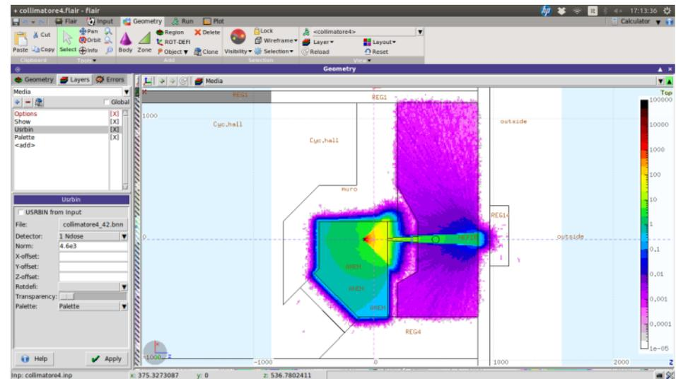
Shielding calculations using Fluka and MCNP is work in progress (courtesy of Stefano Trevisan)
