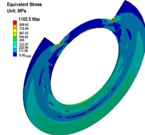
A dynamic model of the stress induced by the thermal expansion is being developed.
