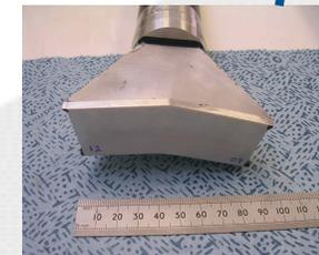
**YAP (YAIO<sub>3</sub>) scintillator** => both the time of flight and the energy E1 of the absorbed neutron are determined when a  $\gamma$  ray is detected
