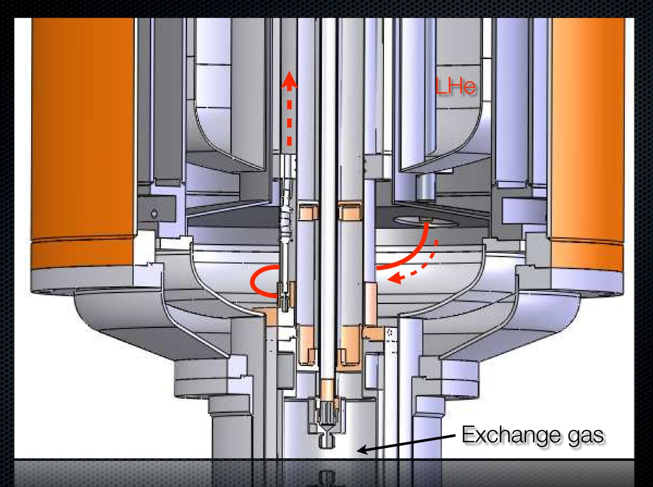
Cryostats (Ø330-450 mm) 1.5 / 2.8 to 320 K Cryofurnaces (Ø330-450 mm) 1.5 to 550 / 650 K Dry cryostats (cryogen-free) 1.8 to 320 K with JT 2.7 to 620 K without JT Sample changers, gonios ?
