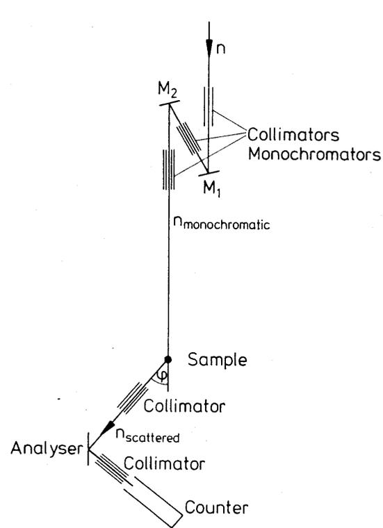
Experimental set-up of a triple axis spectrometer for inelastic neutron scattering (e.g. IN2 of ILL Grenoble).
