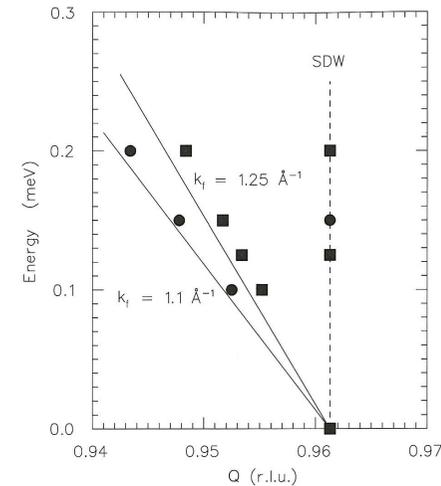
Fig. 6.6. Positions of peaks measured in constant- $E$  scans near a  $(Q_0, 0, 0)$  incommensurate magnetic peak corresponding to spin-wave-density (SDW) order in Cr metal at room temperature. The measurements were performed by Uemura, Grier, and Shirane (1982) at the H9 spectrometer at the HFBR. [r.l.u. = reciprocal-lattice
