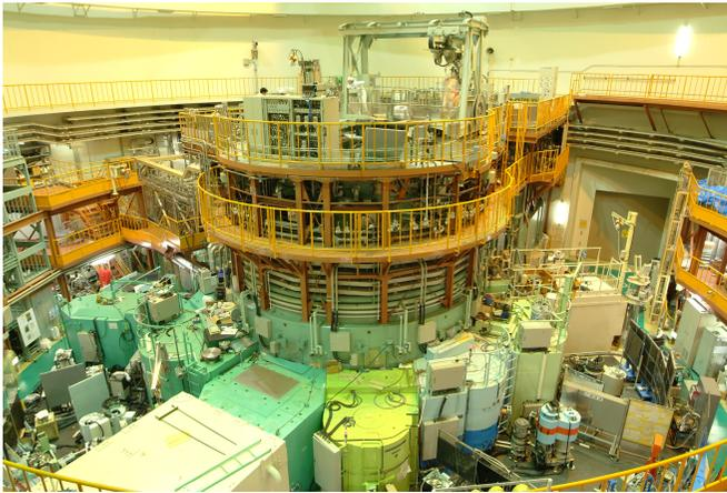
Thermal neutron triple axis instruments in the reactor hall
