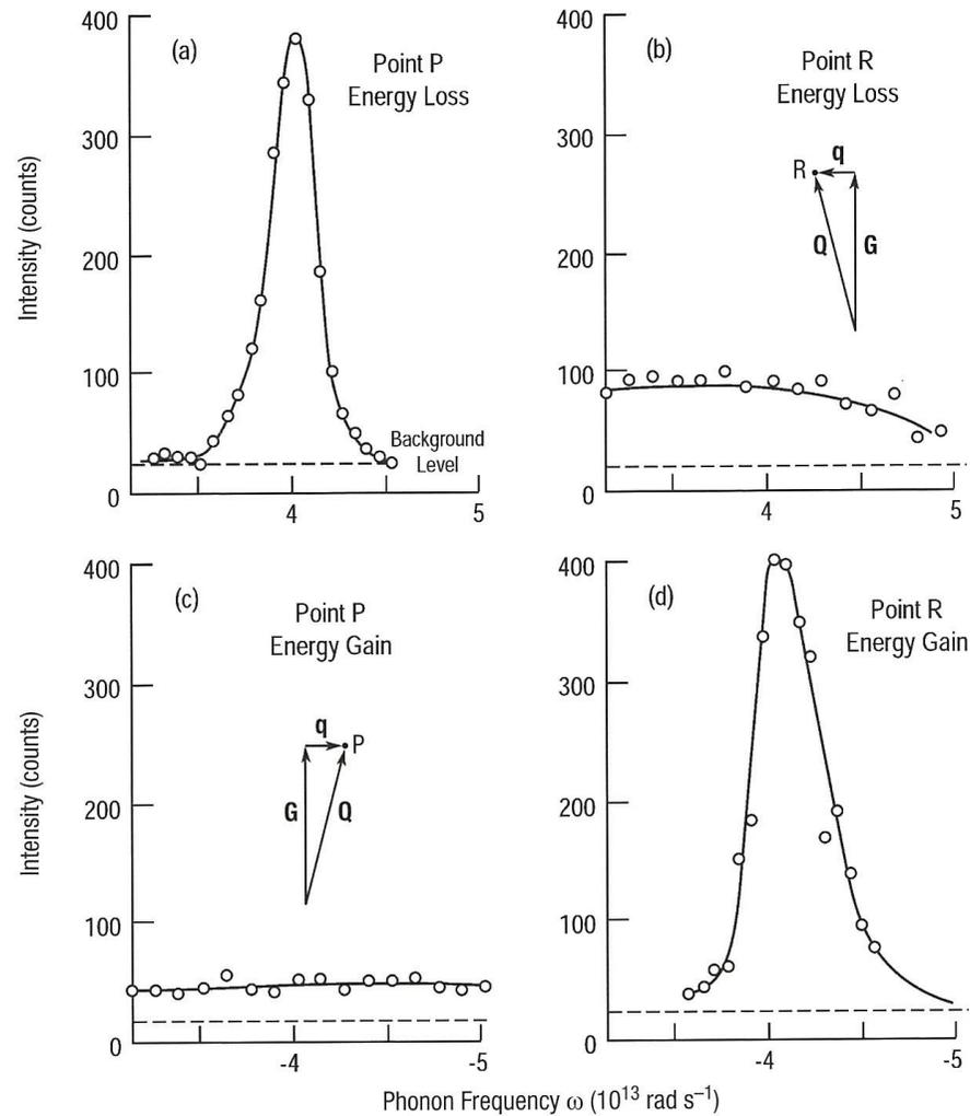
Fig. 4.4. Constant- $Q$  scans of a transverse phonon propagating along a  $[111]$  direction in MgO measured for (a, b) energy gain and (c, d) energy loss at (a, d) focused and (b, c) unfocused positions using a right-handed spectrometer (from Peckham, Saunderson, and Sharp, 1967).
