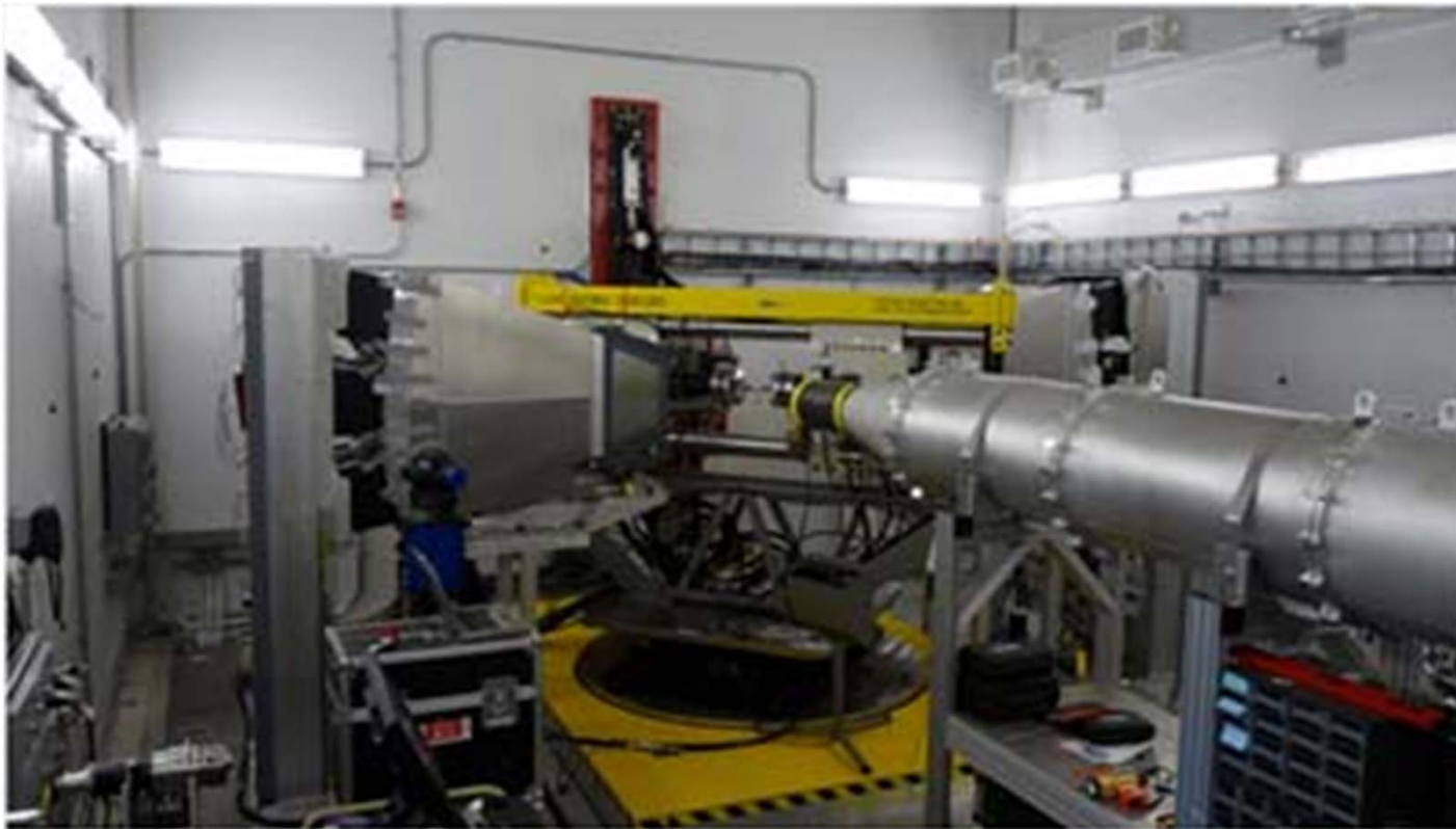
VULCAN instrument (SNS materials/engineering diffraction) with multi-axial load frame
