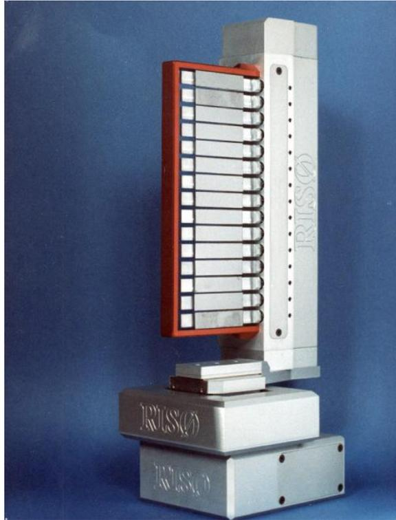
A simple, vertically focusing monochromator produced by Riso National Lab in Denmark comprised of 15 single crystals
