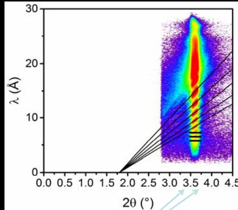
Conventional incoherent summing involves adding the reflectivities from the same wavelengths leading to a loss of resolution
