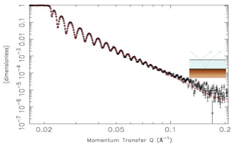
First reflectivity measured on INTER. Nickel/Carbon film (1216  $\text{\AA}$ ) on glass
