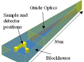
**Figure 4:** An illustration of the possible layout of the Offices beamline (to scale)
