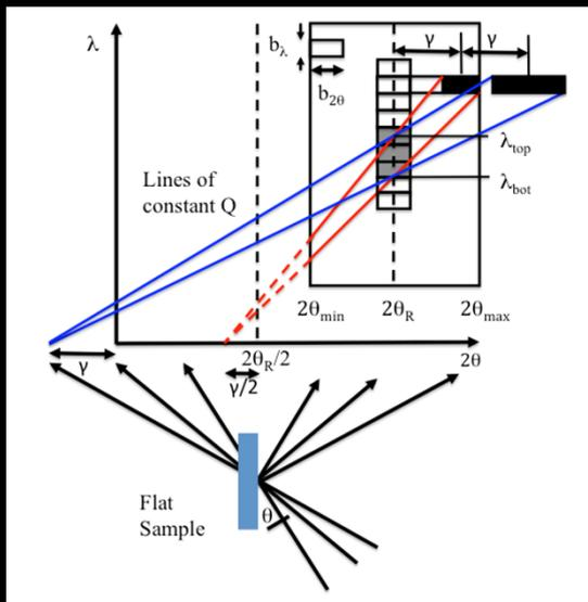
Loop over all pixels and share the reflectivity into all the pixels on a chosen  $2\theta$  line having a virtual wavelength of the same  $Q_z$
