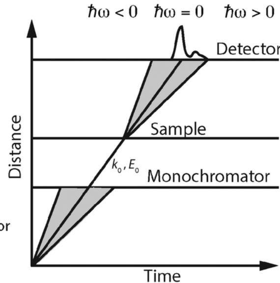
(b) Indirect-geometry spectrometer
