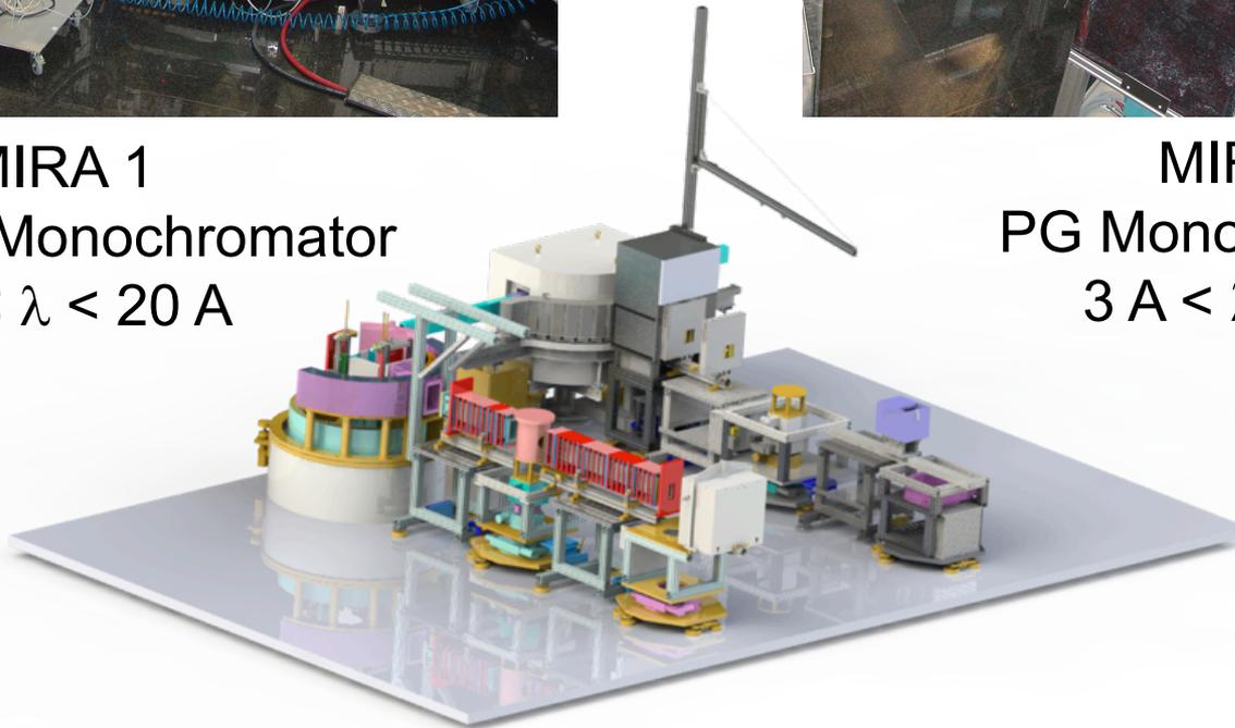
**MIEZE** (Modulation of Intensity with Zero Effort) uses the Neutron Resonance Spin Echo techniques, but the second NRSE arm is missing and the coils are operated at **different frequencies**.
