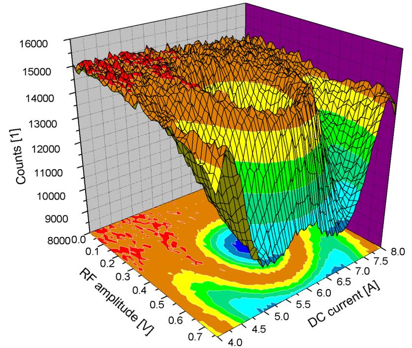
$\pi$  Spin flip at a HF 109 kHz
