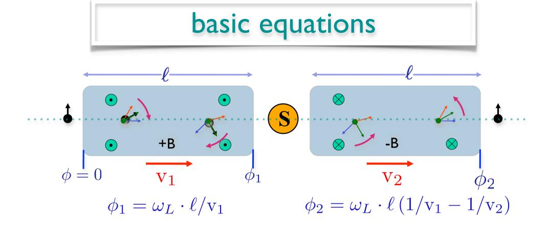
for  $v_1 = v$  and  $v_2 = v + \Delta v \Rightarrow$  $\phi_2 = \omega_L \,\ell \left[ \frac{1}{v} - \frac{1}{(v + \Delta v)} \right] \approx \omega_L \ell \Delta v / v^2 = \omega_L \,t \,\Delta v / v$
