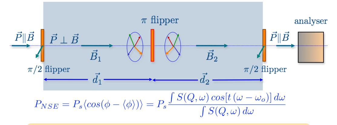
for quasi-elastic scattering  $\omega_{o}$  = 0  $P_{NSE}^{scat}/P_{s} = \Re \left[S(Q,t)\right]/S(Q) = I(Q,t)$
