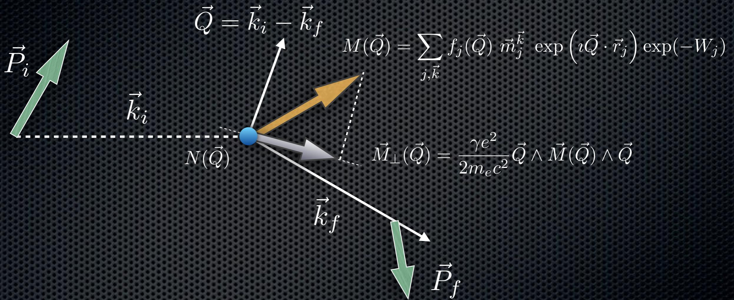
In general, the polarisation of a neutron beam will change both in magnitude and direction upon scattering from a magnetic material.
