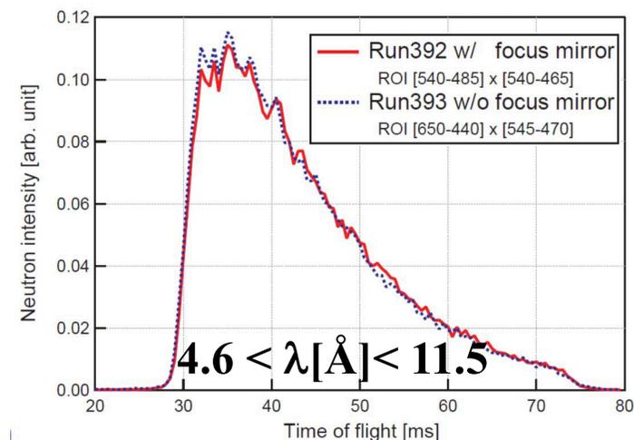
TOF beam profiles for direct beam (blue) and mirror-focused beam (red)
