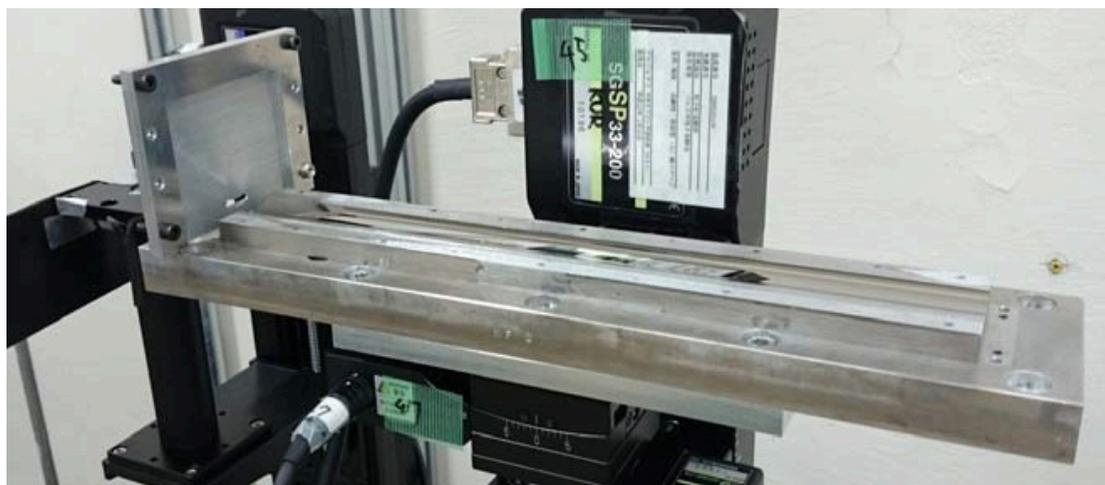
Developed a 2-D elliptical super mirror ( $3Q_m$ ) with 300mm length ( $a = 1250\text{mm}$ ,  $b = c = 20\text{mm}$ ).
