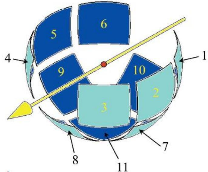
Unlike an image plate set-up the detectors are continuously read-out as a function of TOF allowing spatial overlap to be resolved in the TOF channel while minimising background
