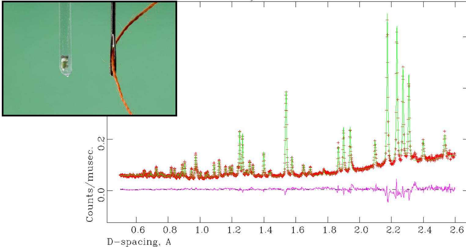
$\sim 1\text{mm}^3$  sample of  $\text{NaNiF}_3$  phase prepared at high  $p$  + high  $T$
