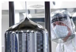
Silicon mono crystal for the semiconductor industry. (Photo: Siltronic)
