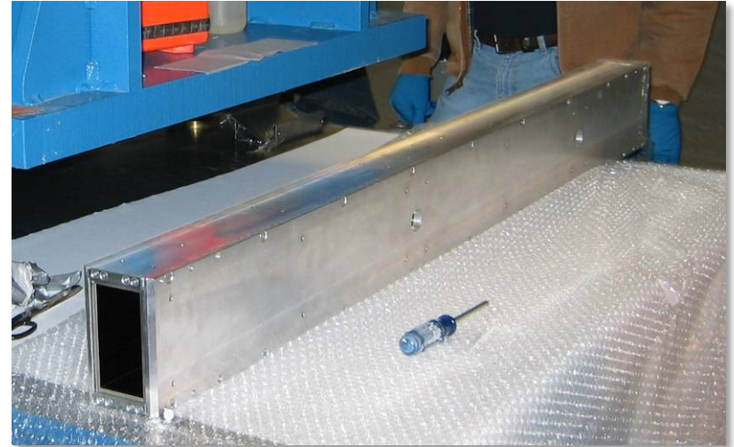
Segment of guide in a steel vacuum housing
