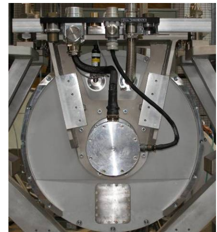
chopper assembled in housing
