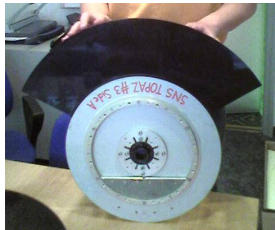
● Neutron Instrumentation III 2 different chopper "disks"
