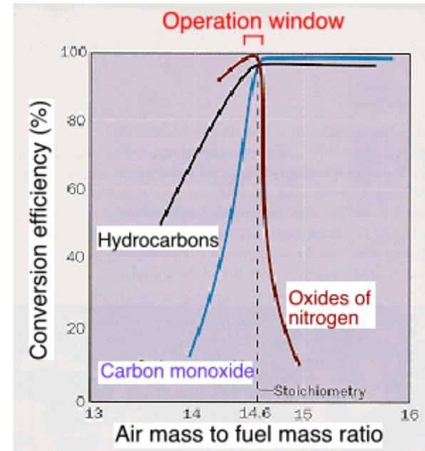
Three-way catalytic converter
