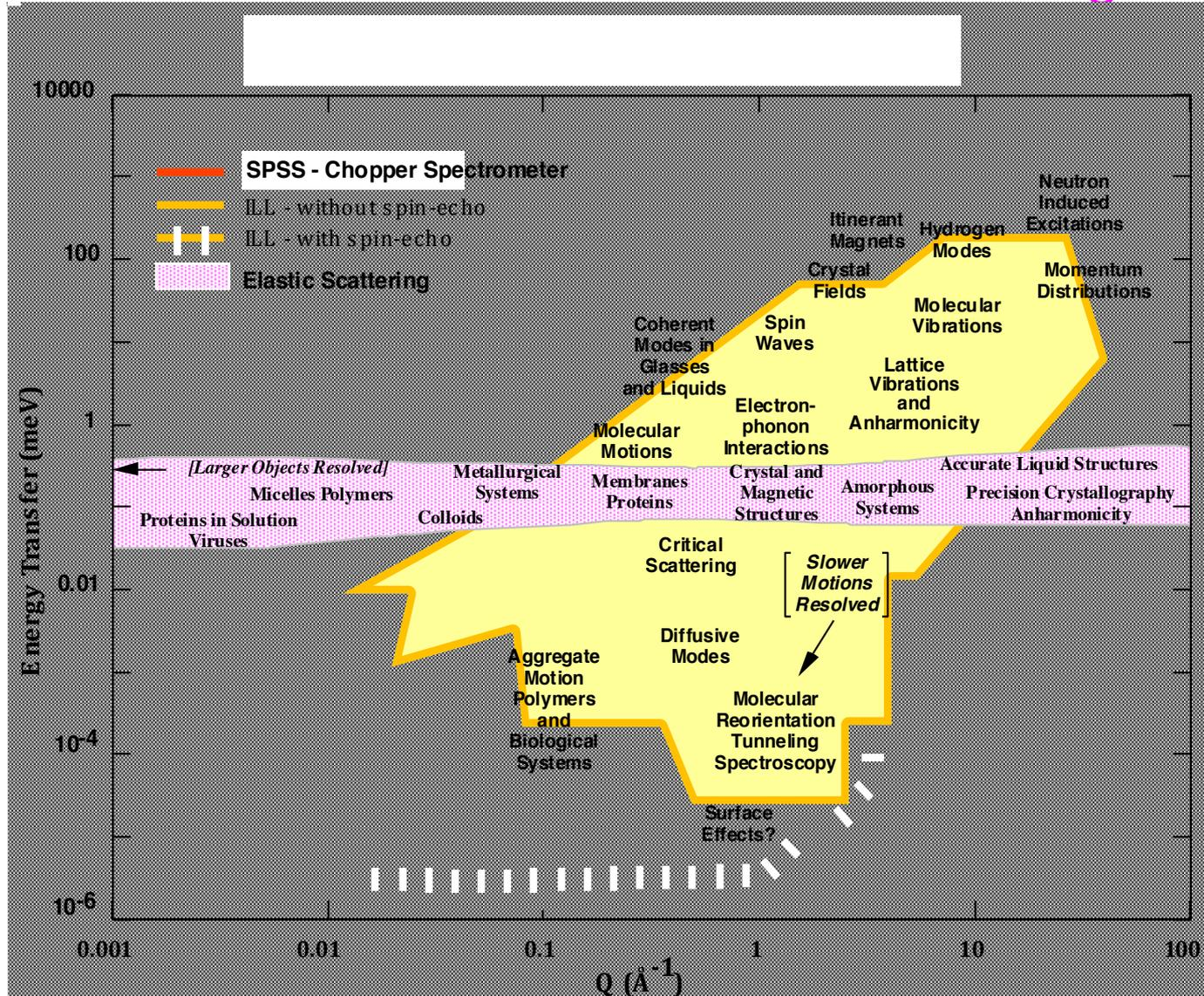
Energy & Wavevector Transfers accessible to Neutron Scattering
