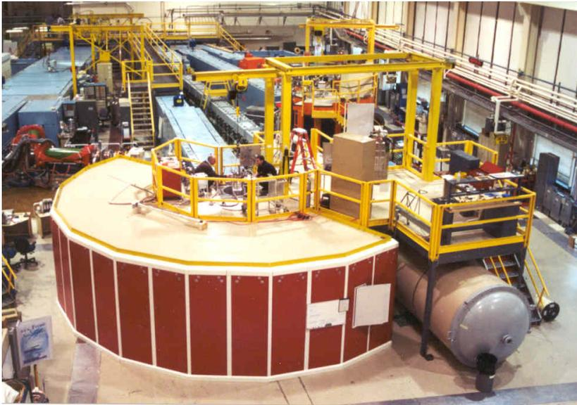
Chopper spectrometer with pulsed monochromatic incident neutron beam and time-of-flight energy analysis
