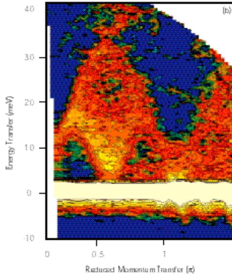
CuGeO<sub>3</sub> is a 1-d magnet. With the unique axis parallel to the incident neutron beam, the complete magnon dispersion can be obtained
