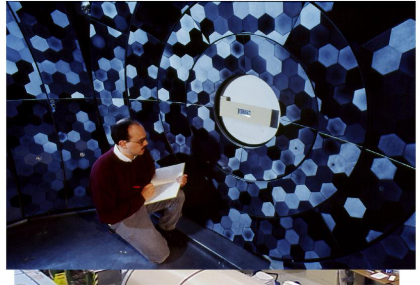
Backscattering spectrometer with polychromatic incident beam and energy analysis by crystal analyzer
