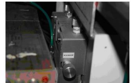
Fig. 17: scheme (left panel) and picture (right panel) of the adjustable slits.
