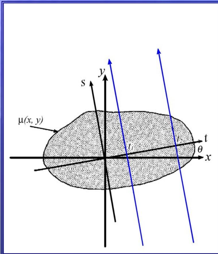
The ray passing through the point  $t_1$  will be attenuated by the interaction with the sample and the measured intensity will be:
