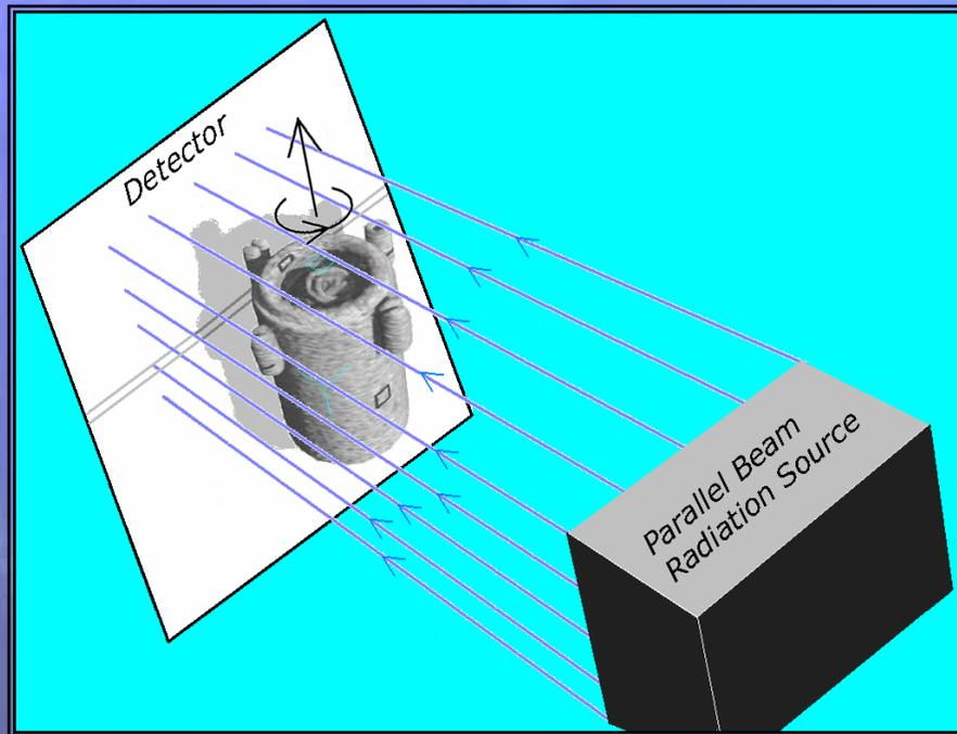
A "*Parallel Beam*" radiation source "*illuminates*" the sample...
