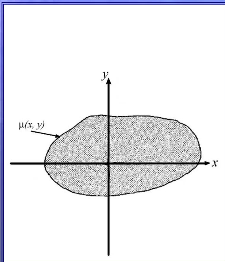
Neglecting other effects (such as scattering, *beam-hardening* etc.) the incident radiation intensity,  $I_0$ , is tied to the transmitted (measured) intensity,  $I_m$ , by the *Beer-Lambert law*:
