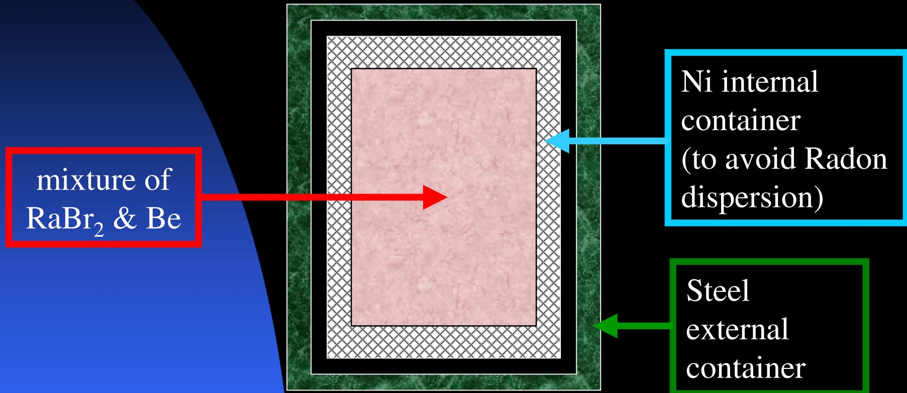
Typical use: detector tests
