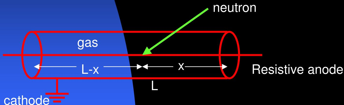
**Measuring the delay between the 2 signals
